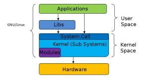
Figure: GNU/Linux System Architecture
