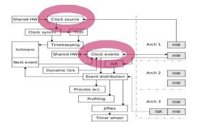
Figure: Linux Time System With hrtimers
