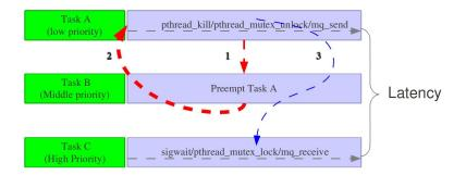
Figure: Kernel Latency of Non-determinism Priority Inversion
