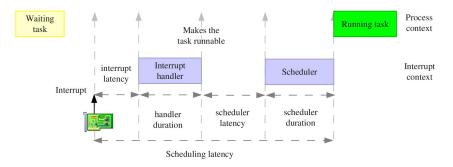
Figure: Kernel Latency of Asynchronous Events
