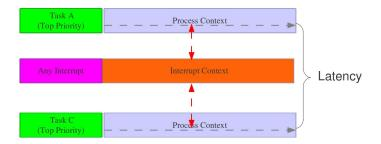
Figure: Kernel Latency of Interrupt Handler Inversion
