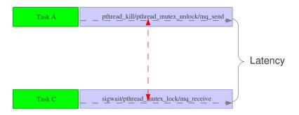
Figure: Kernel Latency of Sync, Mutex and Communication
