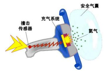
Figure: Control System for Airbag of Car
